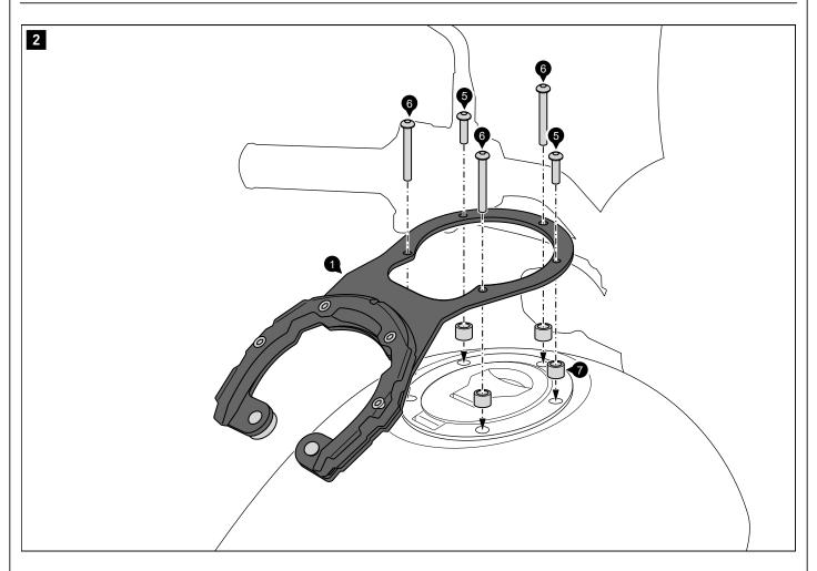
Remove the original screws from the attachment points shown. Screw the mounting bracket (1) to the vehicle. **AWARNING:** Use a liquid threadlocker!
