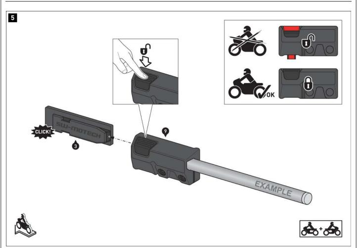
Slide the plug connectors (9/10) onto the connector mounting rails (3/4) on
