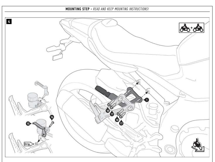
$\triangle$  **NOTE:** This paragraph does not apply to the MT-10 vehicle model. Remove the brake fluid reservoir from the right passenger footrest holder. Then screw the brake fluid reservoir together with the angle bracket (15) and original nut onto the inside of the passenger footrest holder. Tighten the screw (16) as specified in the mounting instructions.
